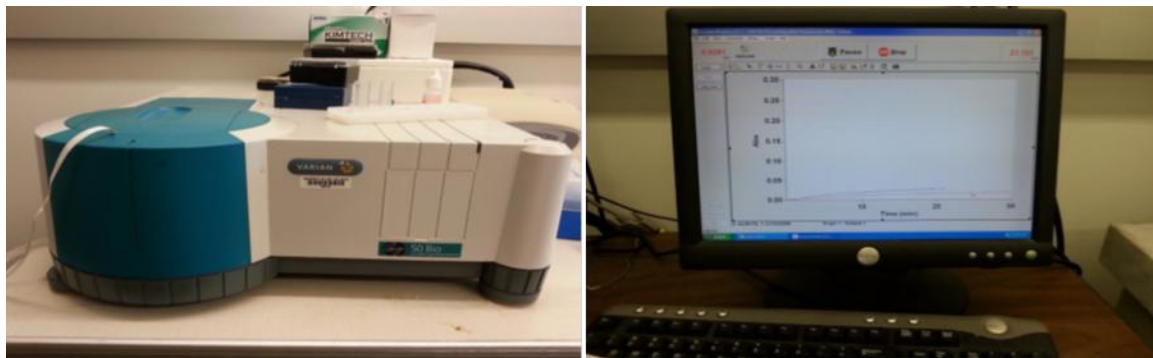
Figure 3.5 UV-Vis spectrophotometer and connected computer used to study the fluorescein release from np-Au
